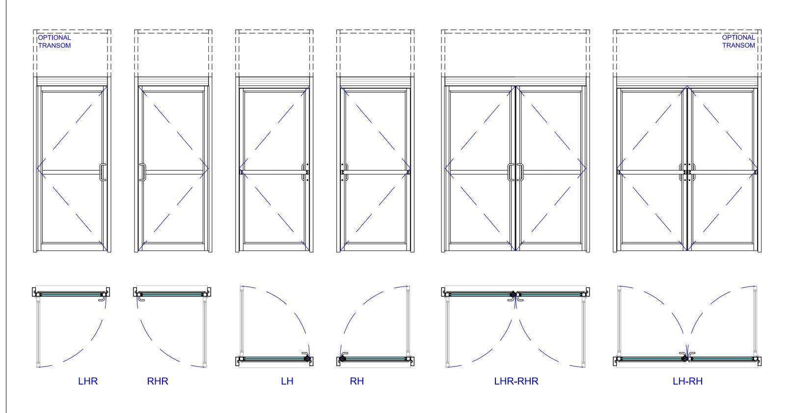
SERIES 8700 OVERHEAD CONCEALED SWING OPERATOR WITH ISOLATED PIVOT (BUTT, OFFSET, CONTINUOUS)
